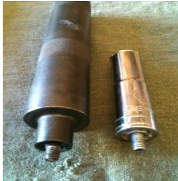
1. Grind or file the barrel adjuster bolt to fit into the square drive end of the socket.
