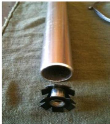
2. With a road style brake cable laced through the center hole, we installed a star fangled nut from a 1" threadless headset into the bottom of the seatpost. The brake cable bead is too large to pass through the center hole of the star nut and will limit the seatpost from moving any higher than the cable length dictates.
