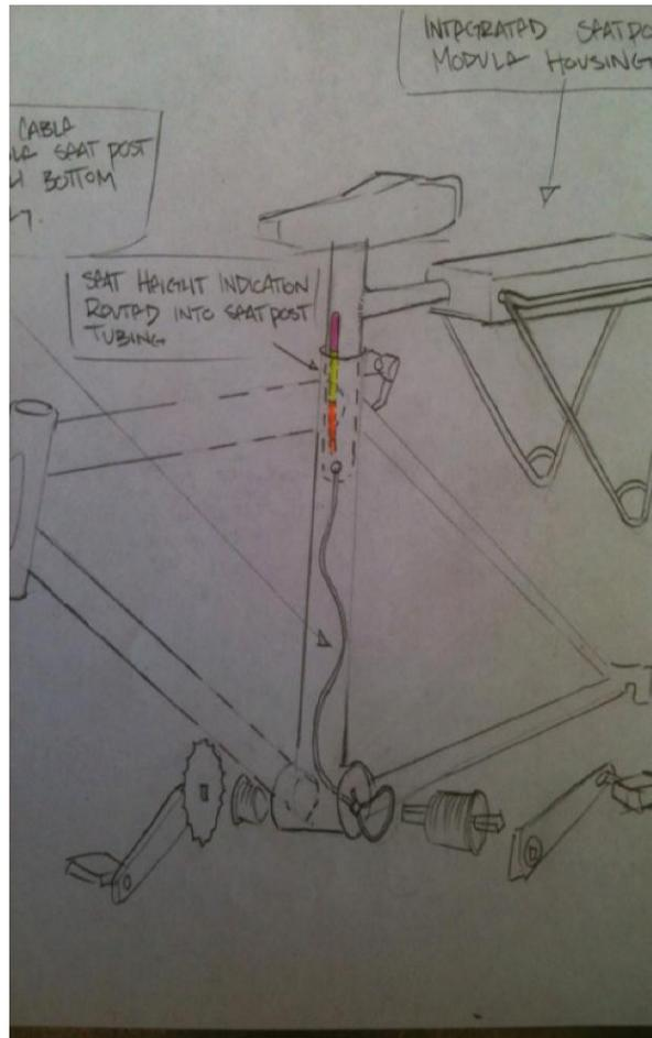
1. The Breezer Uptown Fleet bicycles used for the OBI pilot were equipped with 27.2mm (od) seat posts.
